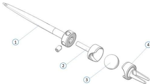
**Figure 2.** Intraosseous DRUJ prosthesis components are: 1- Proximal stem, 2-Locking segment including proximal concave unit, 3- Globe, and 4- Distal stem including distal concave unit.
