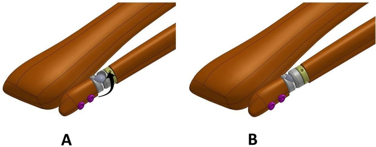
**Figure 3:** By turning locking segment 180 degrees around its longitudinal axis (A), the globe will be locked (B).
